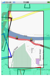
Figure 2: A screenshot showing the “sonification border” used to control the sonification in EdgeTouch.
