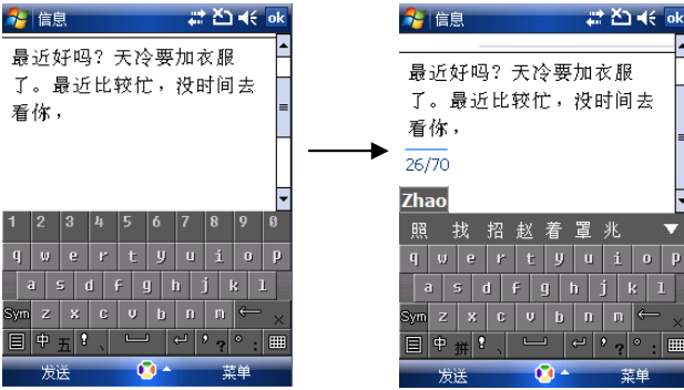
b. the QWERTY keyboard: A pinyin mark is complete by entering its alphabets one by one with the keyboard.
