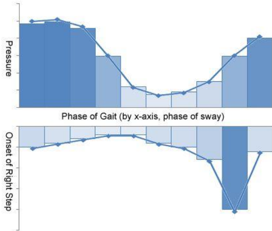
Figure 3. Top: Summation of pressure readings by phase of gait. Bottom: Summation of right step events by phase of gait. A clear correlation exists, thus we can accurately map phase data to phase of step.
