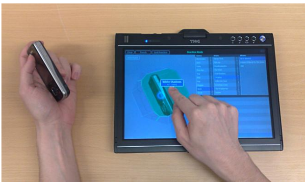
Figure 3. The prototype in use. The user is dragging a song from the browser to the map surface.
