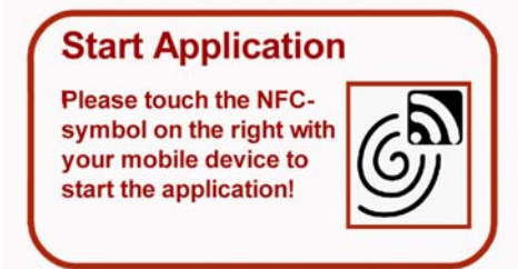
Figure 4. Dedicated start-tag with an enlarged NFC-symbol to initiate interaction with a tagged physical object
