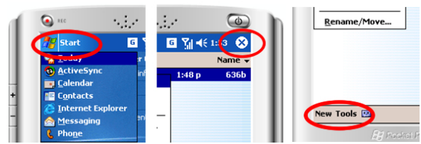
Figure 2 Mobile applications are mostly replicas of their desktop versions in which targetable items can occur in unreachable or difficult to reach areas of the device when using one hand.
