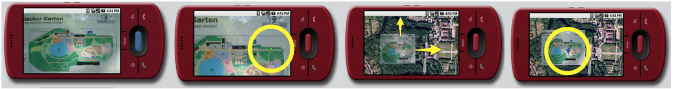
Figure 7: The “Smart Alignment” approach: User takes a photo of a public map and connects the ‘YOU ARE HERE’ dot position to his actual location (the left images, the ‘YOU ARE HERE’ is marked with a yellow circle). After that the photo is overlaid on a digital map and the user can adjust it by scaling it (right). This can be done by using the standard 4-direction joystick (as indicated with the yellow arrows). After completion of this approach the user can use the photo for navigation - the user’s position is indicated with a blue marker (marked with a yellow circle right).
