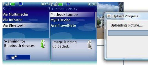
Figure 4. Uploading a picture from the phone to the laptop with standard Bluetooth
