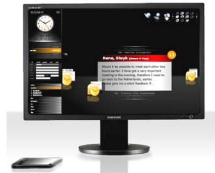
Fig. 5. As the mobile device connects to an external periphery with a larger real estate, the elements of the GUI re-arrange to accommodate the different affordances of the desktop display.
