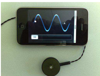
Figure 1: The example application runs on an iPhone with a C2 tactor attached to the audio out port for feedback.
